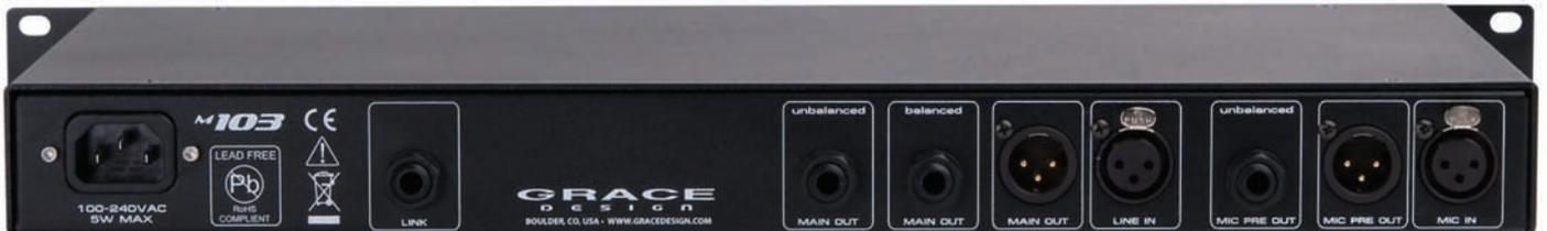
The m103's rear-panel layout lets it operate as either a single channel strip, or as a mic preamp and a separate line-level eq/compressor with makeup gain.
