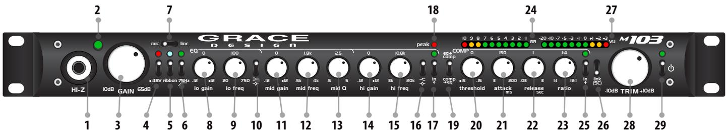
1. **1/4 inch TRS instrument HI-Z input** - Designed to accommodate a wide variety of high impedance input sources, making the m103 an excellent choice as a DI instrument input.
