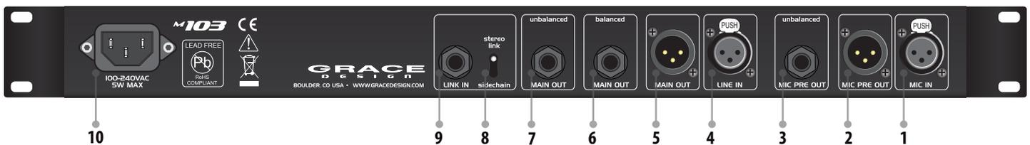
1. **MICROPHONE INPUT** - The XLR microphone input connection, wired with pin 2 positive, pin 3 negative and pin 1 ground. 48V phantom power, when used, is supplied on pins 2 and 3.
